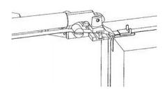
Holding the shear lever with the right hand, push the tension lever back and forth in a full arc with the left hand to tighten the strap.
